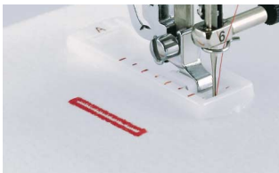
4-STEP AUTOMATIC BUTTONHOLER
